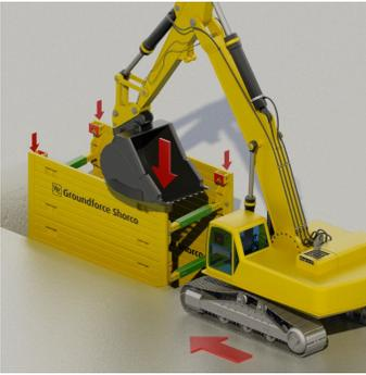
Continue the dig / push process until the required excavation depth is reached.
