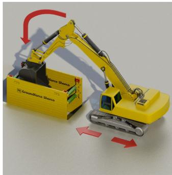
Remove soil from within the base of the excavation.
