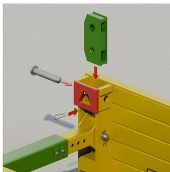
Insert the panel connector cassette and secure with a pin and 'R' clip.
