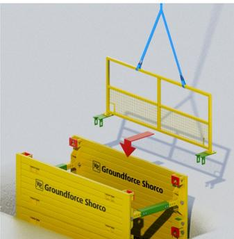
Edge protection barriers are fitted by using a sling and lowering onto the top panels from above.
