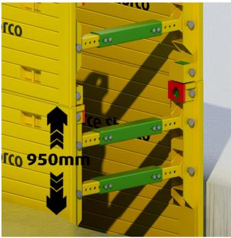
Once the **lower box** is 950mm above ground level, the upper box can be removed.
