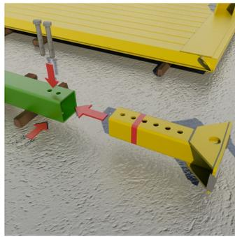
Adjust the assembled strut, if necessary, to suit the excavation width and secure using 2No. Pins and 'R' Clips per Rocker (4 per strut). **Note: Struts must only be adjusted while horizontally orientated.**
