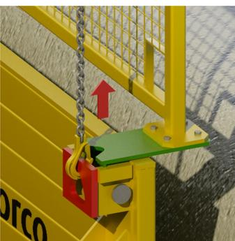
Using a single heavy duty chain attached to each corner of the box, lift by no more than 150mm each time. **Note:** access the lifting point through the opening in the handrail panel.
