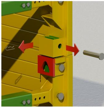
Remove the pins and 'R' clips to release the top box.
