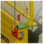
Using a single heavy duty chain attached to each corner of the box, lift by no more than 150mm each time. **Note:** access the lifting point through the opening in the handrail panel.
