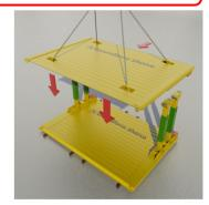
Using the four handling points, lower the second panel onto the struts.
