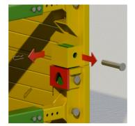
Remove the pins and 'R' clips to release the top box.
