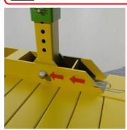
Fit an 'R' clip through the pin on the inside
