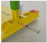
After adjusting the struts to the required width, Fit a strut into the strut rocker housing (See safety note below) Insert a pin and 'R' clip. Fit the pin from the outside as shown.
