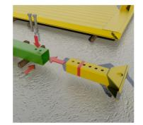
Adjust the assembled strut, if necessary, to suit the excavation width and secure using 2No. Pins and 'R' Clips per Rocker (4 per strut). **Note: Struts must only be adjusted while horizontally orientated.**
